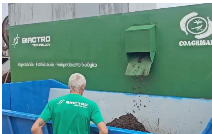
Class A amendment discharged at the outlet of the biocatalysis module.
